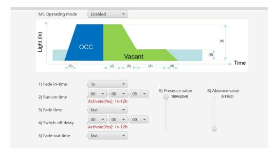
(1) Fade in time: this means the time that the destined DALI luminaires take to fade from current state to the configured state when the movement detected and the room is occupied.
